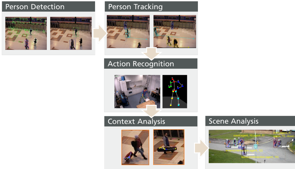
Figure 1.1: This figure depicts the pursued pipeline from images to semantic scene descriptors at the VCA group at the Fraunhofer IOSB.
