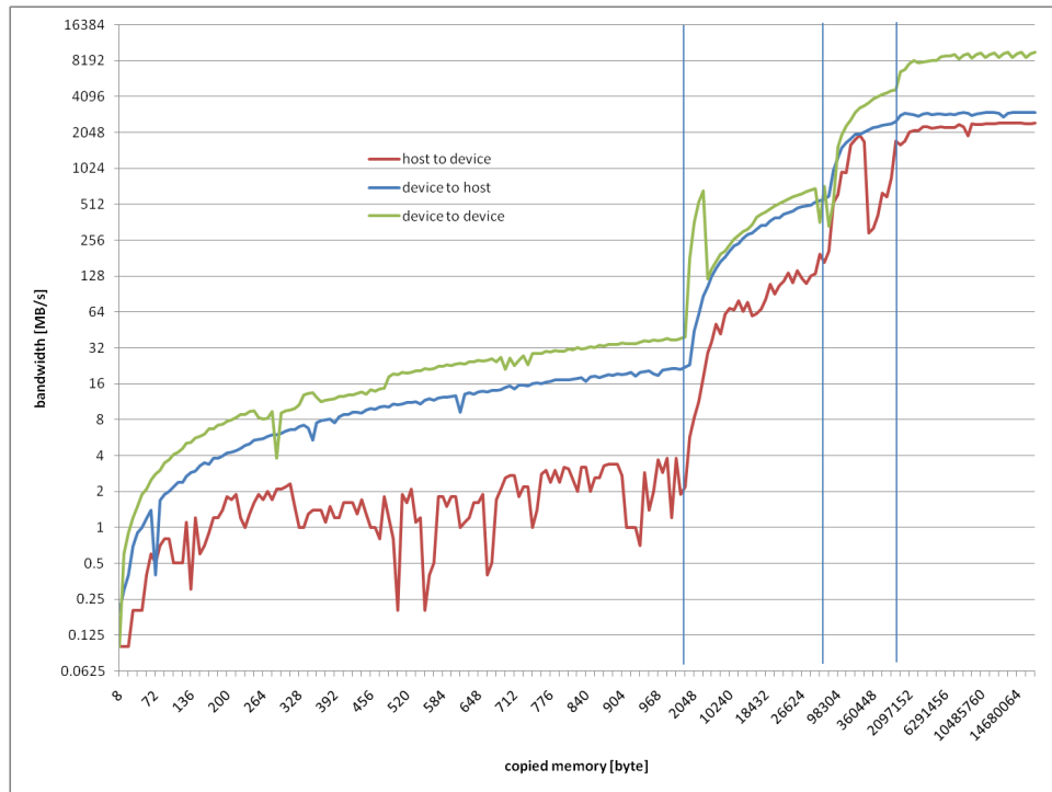
Figure B.10: Bandwidth of memory transfers from host to device, device to host and device to device. The vertical lines show an increasing increment of transferred data.
